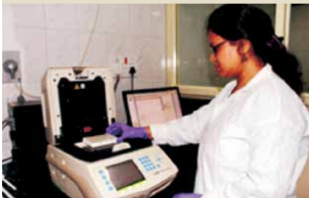
Real time PCR for the detection of viral copy number in JE infected embryo
